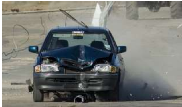
Passively safe post (140mm dia) minor damage to bonnet/bumper vehicle still driveable, low deceleration.
