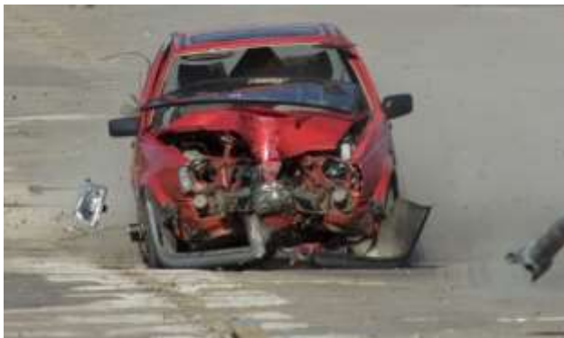
Traditional post (114mm wide base) vehicle badly damaged, rapid deceleration
